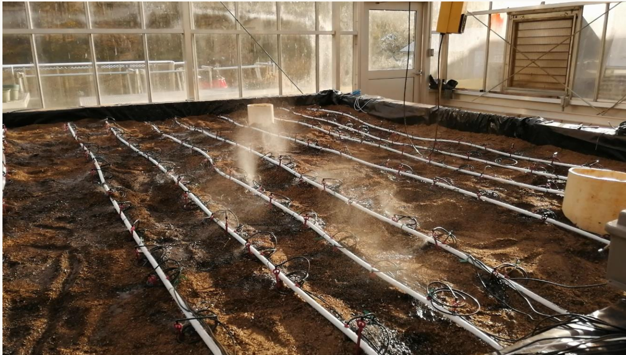
Volumetric water content regulated with 128 sensors to control 128 sprayers
