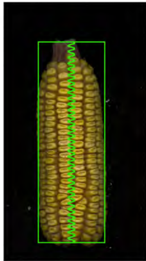
Major and minor axes measured for each kernel (above). Fourier transform of the ear (left) measured the average kernel length in the axial direction. Together, these two measurement modes determine the three principal dimensions of the average kernel on an ear.
